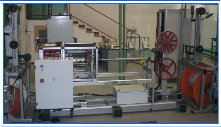
The line, composed by pay-off, taping head, capstan and take up can be used to tape cable up to 10 mm diameter. All the line is controlled by digital bus for the synchronizing of all motors and drives. All the parameters of tape tension can be adjusted by recipes settable through touch screen.
